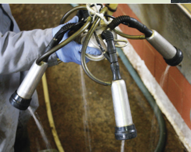
Action – the flushing system uses about a pint of fluid and takes 30 seconds to complete the cycle.
