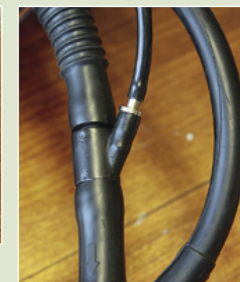
Left: Cluster with AirWash fitted. Flushing liquid passes into the liners via the small pipes joining the milk tubes. Middle: Here's the junction point between the small milk tube and flushing pipe. The junction has a one-way valve to prevent vacuum stability being compromised. Right: The flushing sequence of fluid and air is controlled by this box. Up to five rinse and air blasts are typically used within each rinse cycle.
